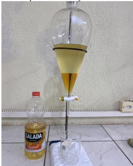
Figure 2: Decantation process of methyl biodiesel from sunflower oil.
