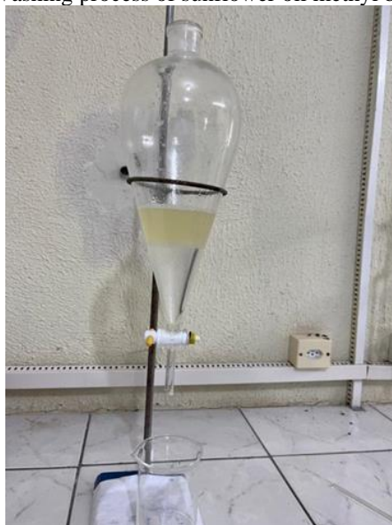
Figure 6. Washing process of sunflower oil methyl biolubricant.
