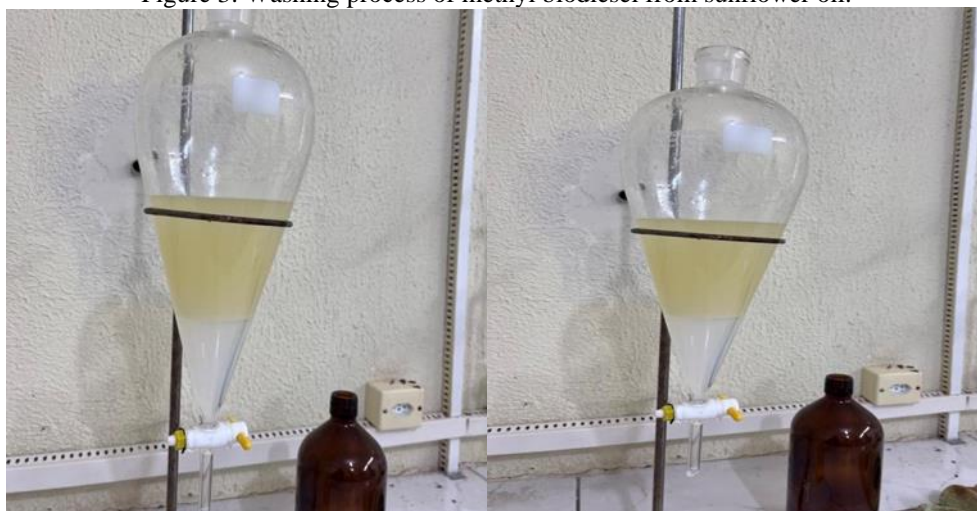
Figure 3: Washing process of methyl biodiesel from sunflower oil.
