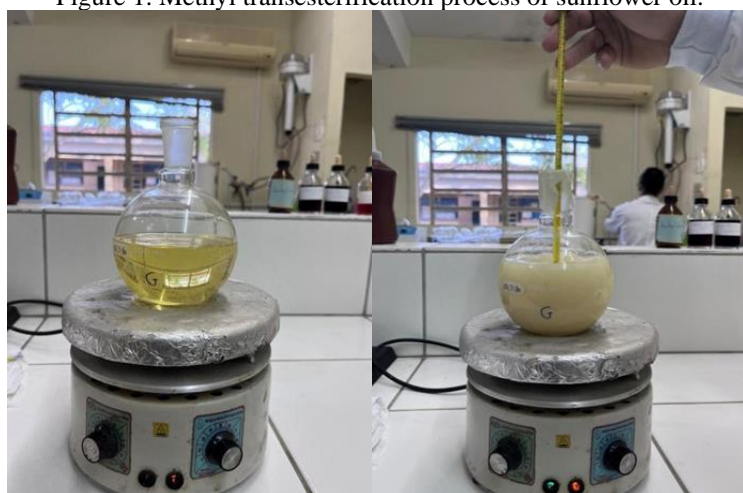
Figure 1. Methyl transesterification process of sunflower oil.
