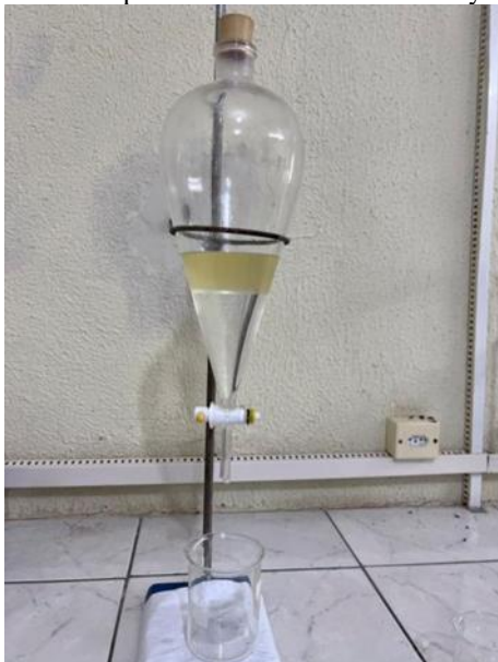
Figure 5: Decantation process of sunflower oil methyl biolubricant.
