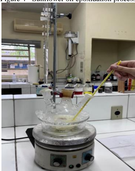
Figure 4 - Sunflower oil epoxidation process.
