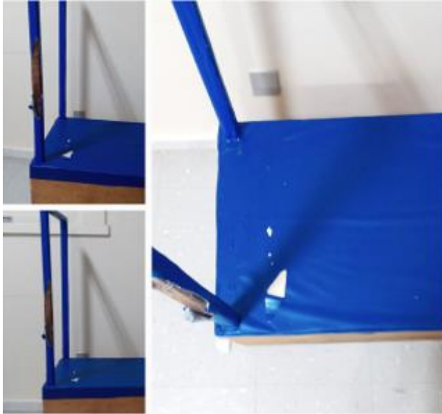
Figure 9 - Wear found on the supports
