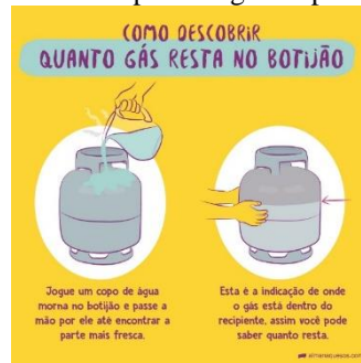
Figure 5 - Example of measurement shape through temperature difference in the cylinder.
