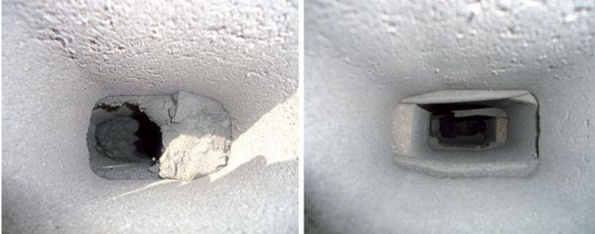
Figure 1 - Using the spoon (left side) and using the tube (right side) to apply mortar.
