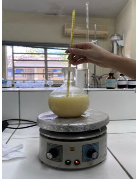
Figure 1. Methyl transesterification process of corn oil.
