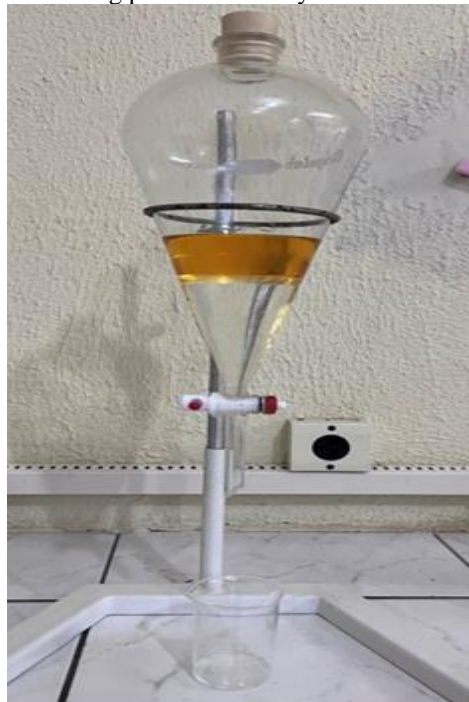
Figure 2: Decanting process of methyl biodiesel from corn oil.
