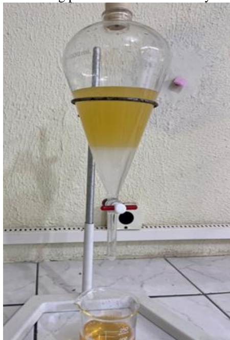
Figure 3: washing process for corn oil methyl biodiesel.
