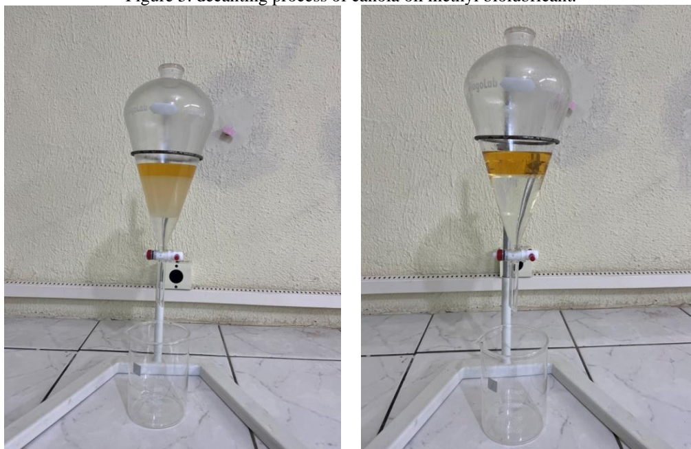
Figure 5. decanting process of canola oil methyl biolubricant.
