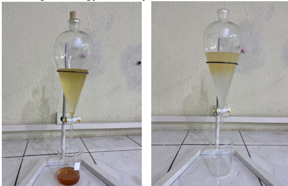
Figure 3. washing process of methyl biodiesel from canola oil.
