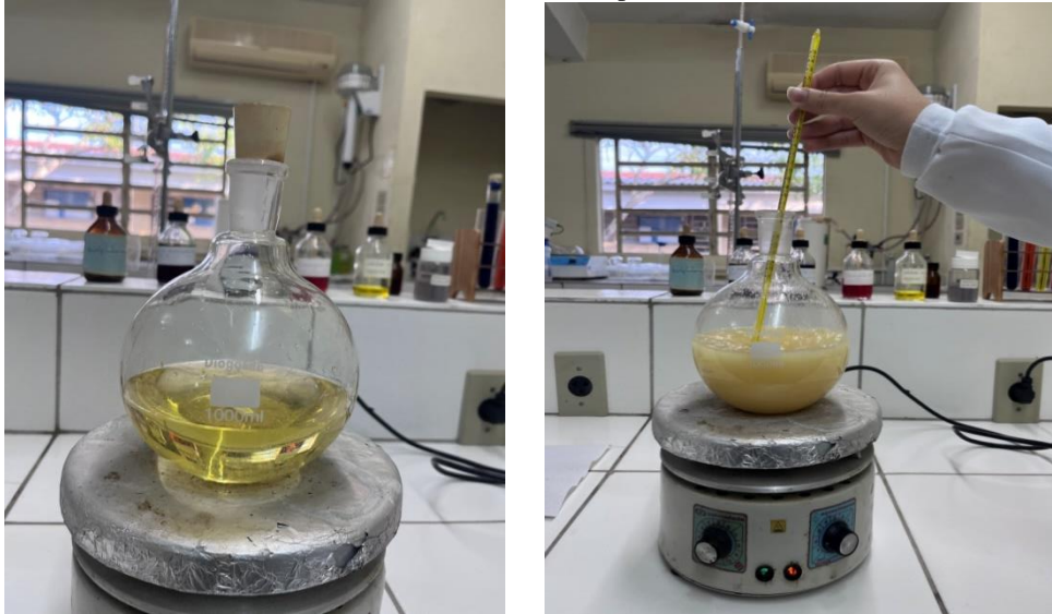
Figure 1. Methyl transesterification process of canola oil.
