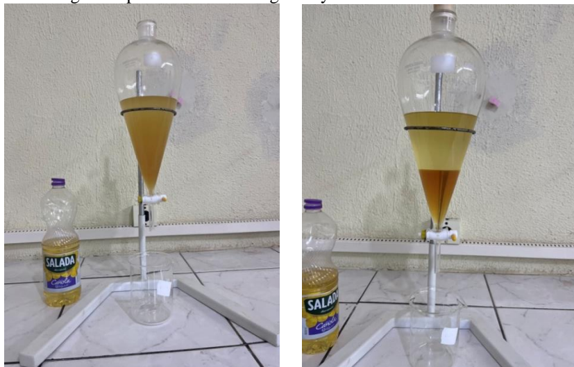
Figure 2. process of decanting methyl biodiesel from canola oil.
