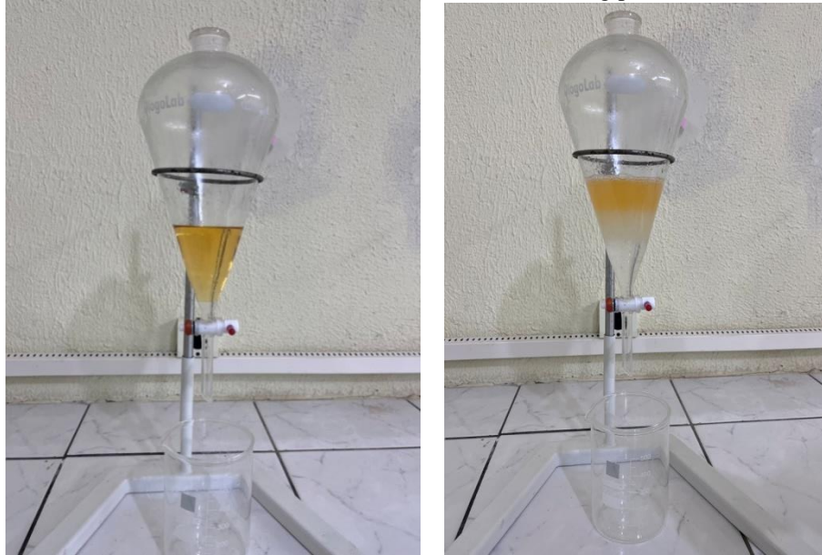
Figure 6. Canola oil methyl biolubricant washing process.
