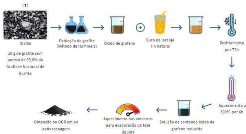
Figure 1 – Flowchart of the methodology for obtaining the reduced OG with apt orange juice (for reduction with inapt orange, an analogous method was used).
