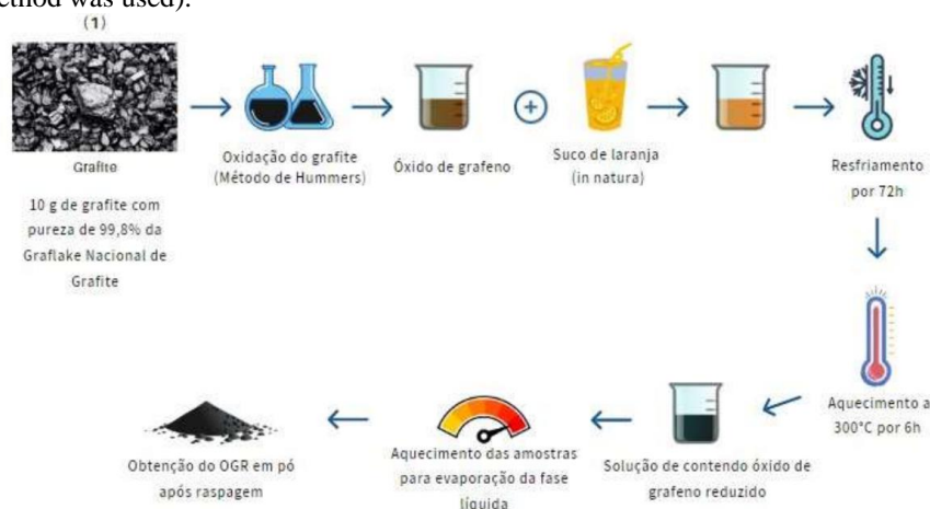
Figure 1 – Flowchart of the methodology for obtaining reduced GO with suitable orange juice (for reduction with unsuitable orange, an analogous method was used).
