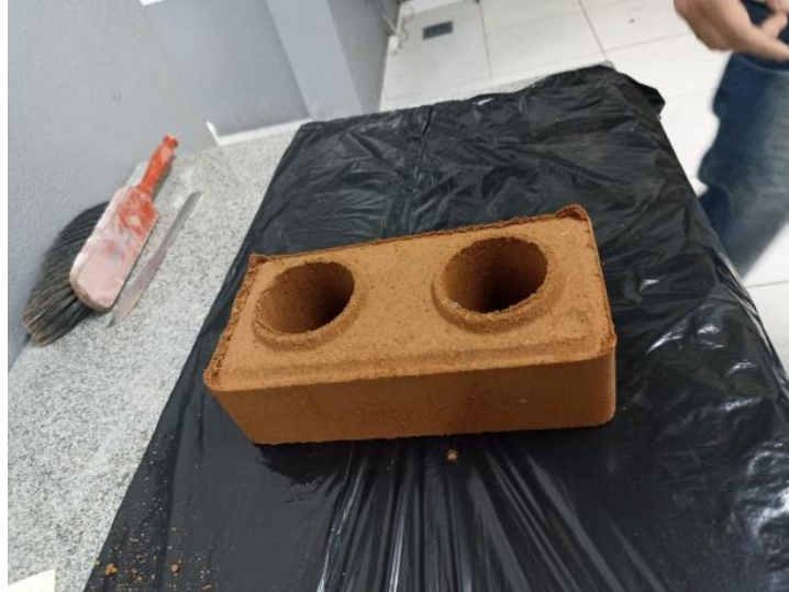
Figure 1: Ecological soil-cement brick manufactured by the authors.
