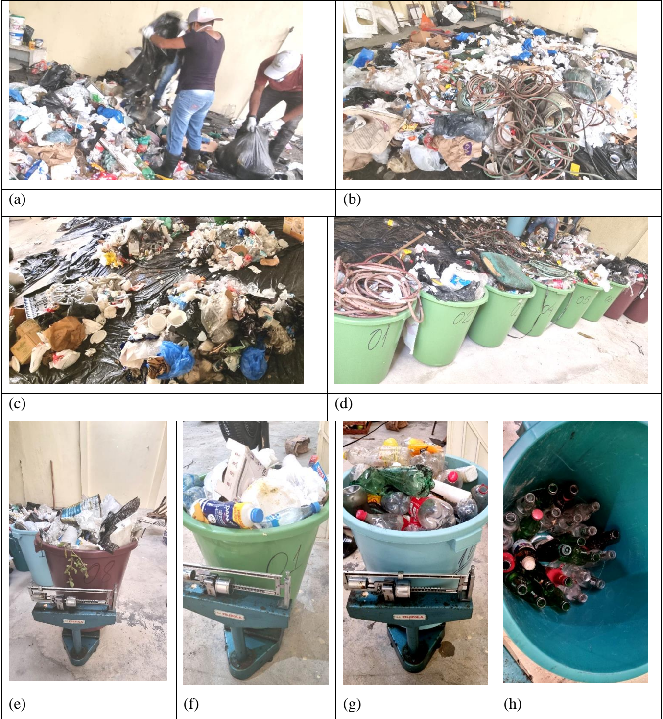
Figure 4. Gravimetry: (a) Removal of waste from plastic bags; (b) mixing of waste; (c) quartering; (d) separation of 1m 3 of waste; (e) and (f) weighing of mixed waste; (g) and (h) weighing of waste separated by type; (i) separation of waste by type; (j) weighing of waste by type.
