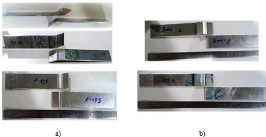
Figure 2: Different views of mode II failure in a joint.
